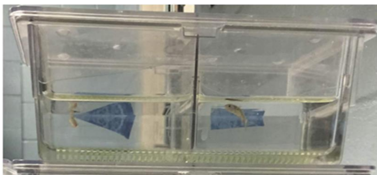
Fig. 9. A zebrafish spawning apparatus is illustrated here. To stop the adult fish from eating the eggs, the mechanism is made to let them fall to the bottom of the tank through a slotted insert
