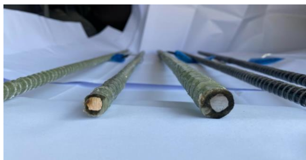
Figure 2. Hybrid steel-GFRP bars [63]
