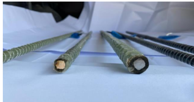
Figure 2. Hybrid steel-GFRP bars [63]
