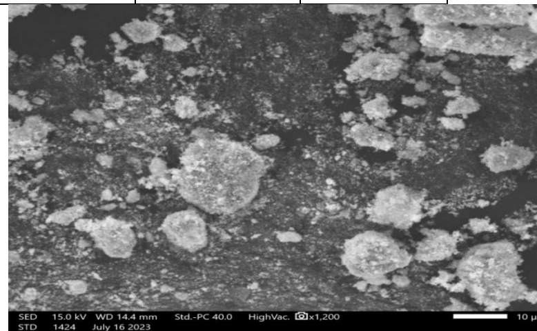
Figure (4): SEM surface image of nanoparticles ZnO powder.
