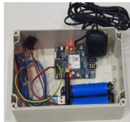
Fig. 4. Tracking System based on SIM-808 Module.
