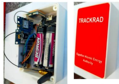
(b) Tracking System based on SIM-800L Module
