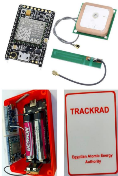
Fig. 5: Tracking System based on A9G Module
