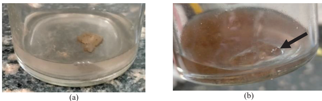
Figure 4 Post cured vitrimer sample S1B1cured220-8 in TFA (a) at the test start (b) swelling of sample after 72 hrs.
