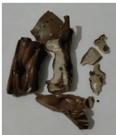
Figure 1. Vitrimer S1 B1 after heating under 220 to 240°C for 8.5 hrs
