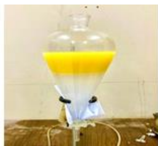
Figure 4. Water washing process (Washed biodiesel).
