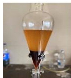
Figure 3. Settling and Separation process (Biodiesel + Glycerol).
