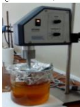
Figure 2. Magnetic stirring with lab mixture: Ultrasonic setup (Transesterification).
