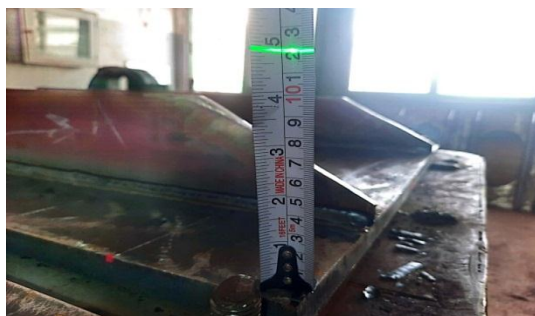
Figure 5. FLG type Laser device evaluating second measuring after constraints released.
