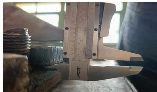
Figure 6. Re-checking the final displacement value using a vernier caliper.
