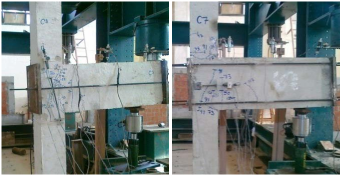
Figure 11. Failure patterns of selected specimens [21].
