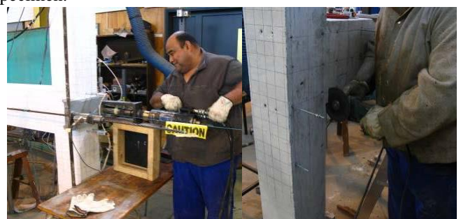
Figure 10. Retrofitting approach (post-tensioning and partial removal of bottom reinforcement) [20].
