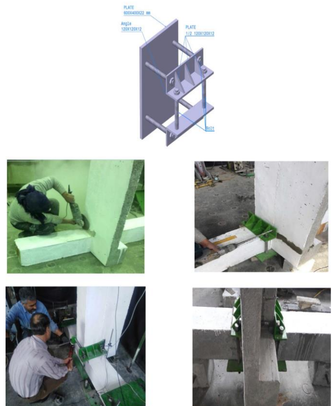
Figure 15. Retrofitted system set up [25], all dimensions in mm.
