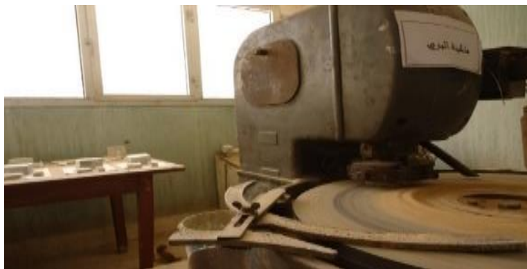
Fig. 3: Machine used for abrasion test.
