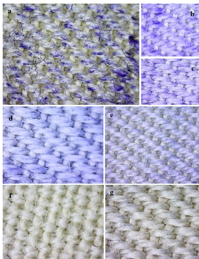
Fig. 13. Microscopic examination of stained control sample (a), the sample treated with agarose 5% and isopropyl alcohol 60% (b), the sample treated with agarose 3% and isopropyl alcohol 60% (c), the sample treated with agarose 3% and isopropyl alcohol 80% (d), the sample treated with isopropyl alcohol 100% (e), the sample treated with the commercial solvent under suction table (f), and the sample treated with the isopropyl alcohol 100% under suction table (g).
