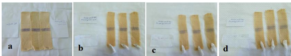
Fig. 11. The samples treated with commercial solvent with agarose 2%. a) before treatment; b) 30 minutes; c) 60 minutes; d) 120 minutes.
