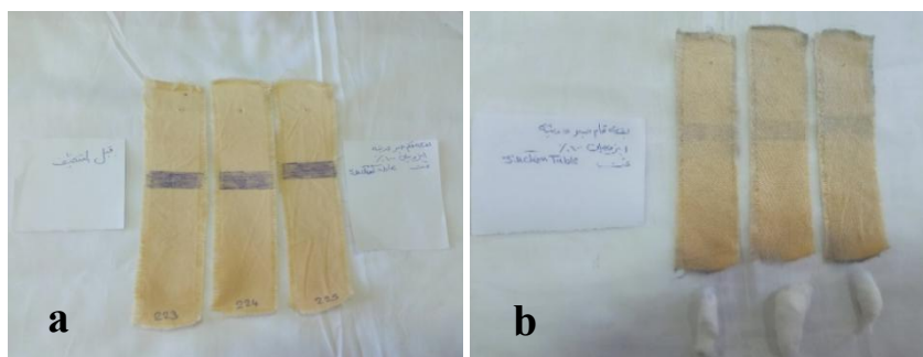
Fig. 4. The samples treated with isopropyl 100% under suction table. a) before, and b) after treatment.
