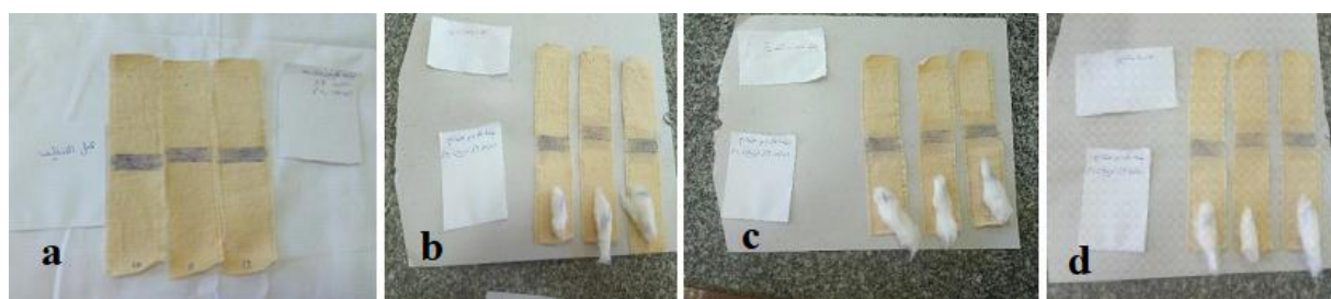
Fig. 7. The samples treated with agarose 3% with isopropyl alcohol 100% treatment. a) before treatment; b) 30 minutes; c) 60 minutes; d) 120 minutes.
