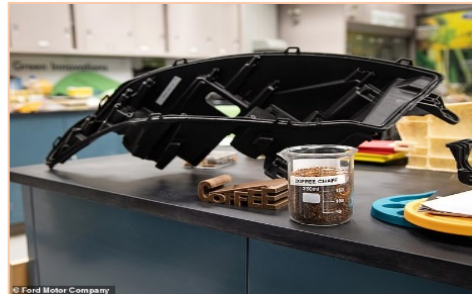
Fig.18: Recycling coffee wastes to produce car parts at Ford factory
