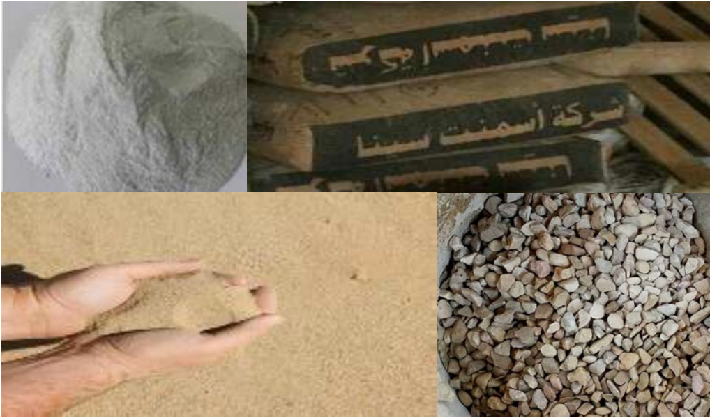
Fig.1. Materials used: Ordinary Portland Cement (OPC), fine and coarse aggregates, potable water, and waste glass powder (WGP).
