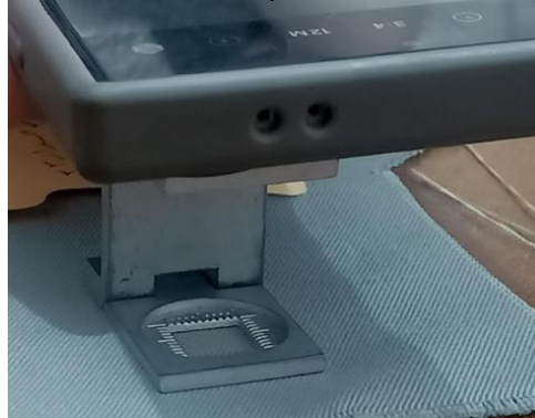
Figure (2) iPhone camera above the lens to take a picture of the fabric
