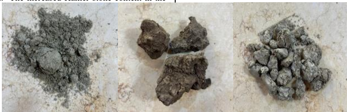
Fig. 2: The dry materials shown from left to right are Nile Silt, Hamar stone, and ash. All four clay batches exhibited good plasticity during forming. However, the higher Nile Silt content in batch 3 reduced its workability, making it difficult to throw on the wheel. Consequently, batch 4 was developed, using equal parts clay and Hamar stone, supplemented with 10% ash recycled
