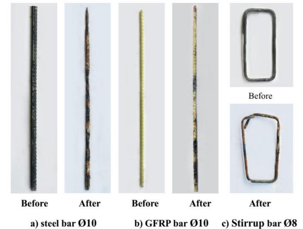
Fig. (11) Steel rebar Ø10 and GFRP bar Ø10 before and after the accelerated corrosion test. Table (6) weight of the reinforcement cage (Kg) before and after the corrosion process.
