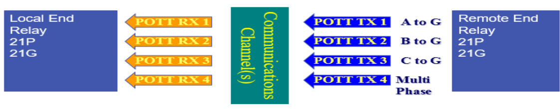
Figure 3: Permissive scheme with IEC 61850 4-bit communication channel
