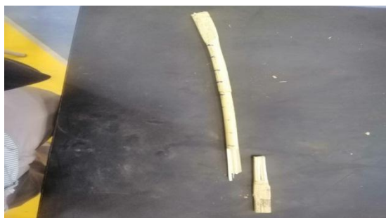
Figure 5. Splitting and Grip Failure (sample-3)
