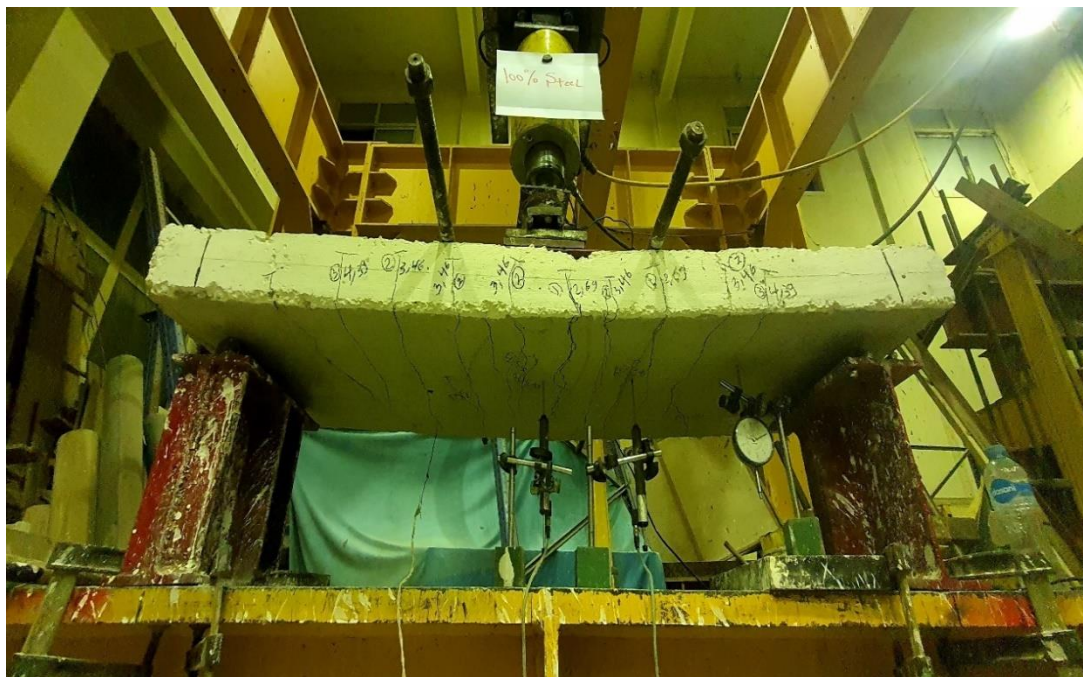
Figure 13. Final Crack patterns for 100% Steel Reinforced Slab (S100-B0) %.
