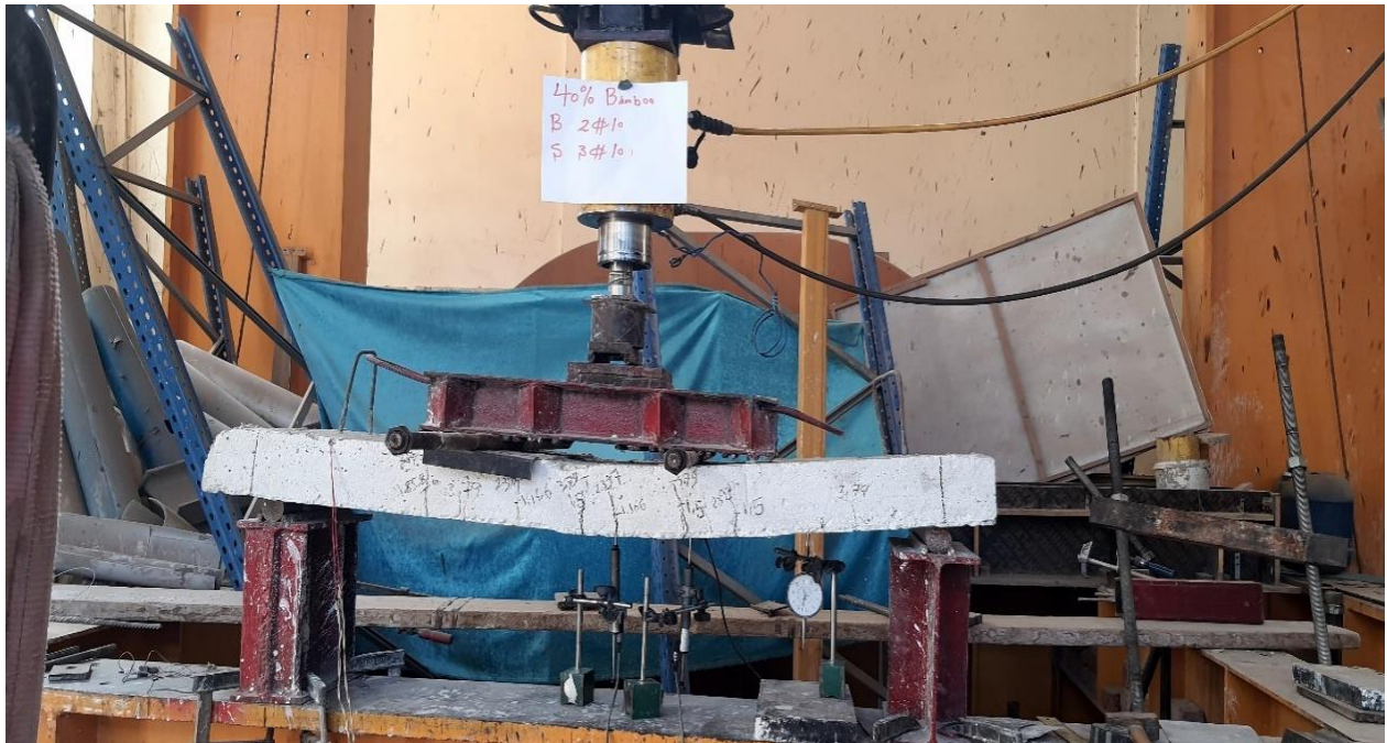
Figure 17. Failure mode for the slab 40% Bamboo (S60-B40) %.
