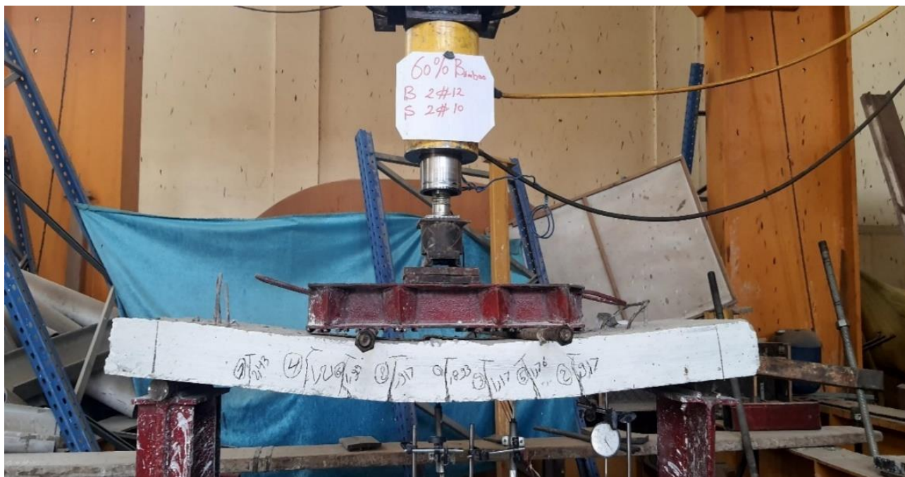
Figure 23. Failure mode for slab Reinforced (S40-B60 12mm) %.
