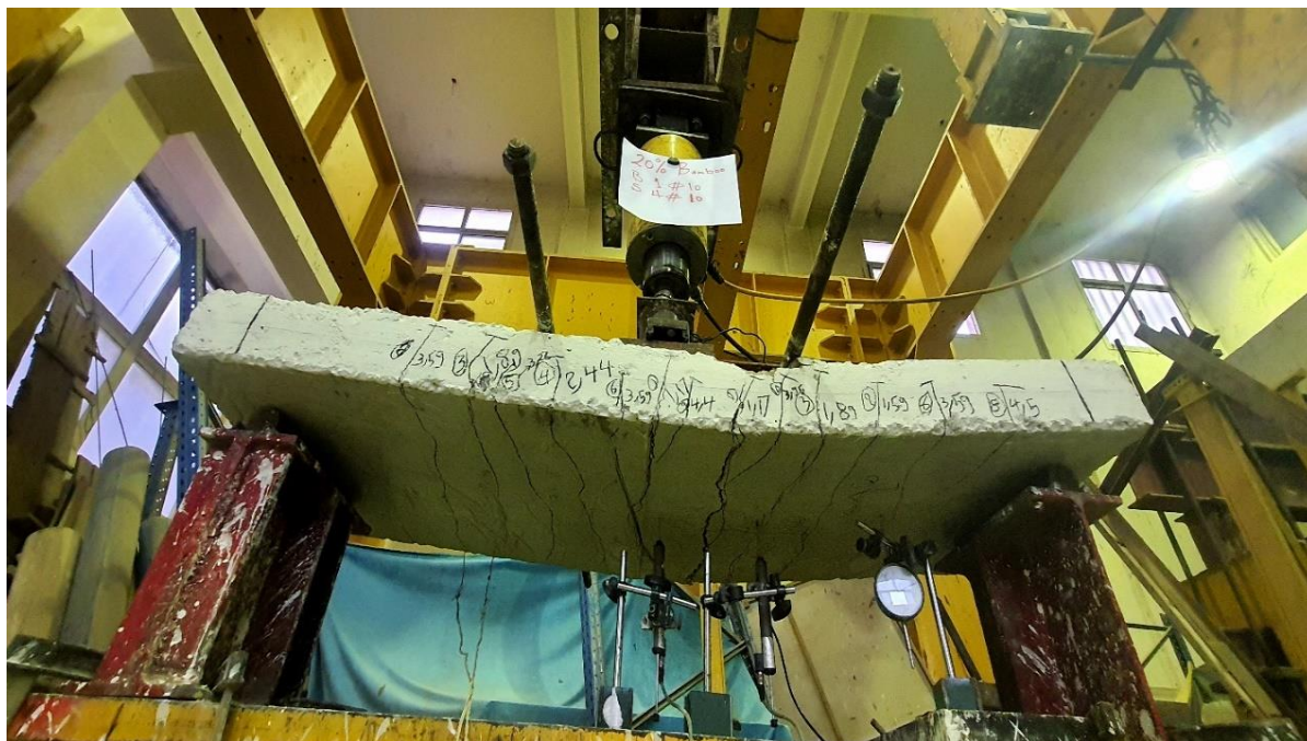
Figure 1. Failure mode for the Slab 20% Bamboo (S80-B20) %
