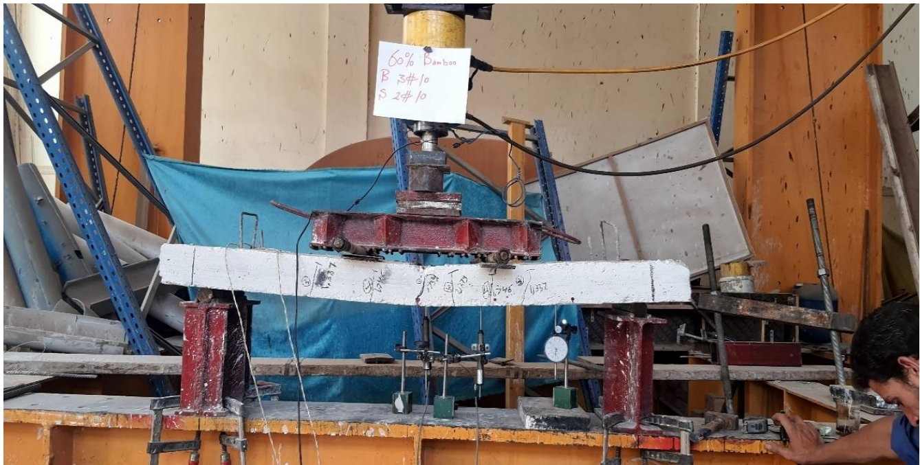
Figure 20. Failure mode for the slab 60% Bamboo (S40-B60) %.
