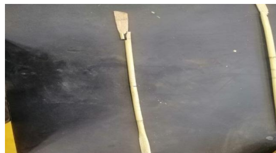
Figure 6. Splitting and Grip Failure (sample-4)
