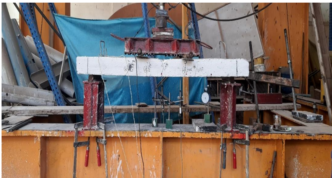
Figure 28 Final Crack patterns for 80% Bamboo Reinforced Slab (S20-B80) %.
