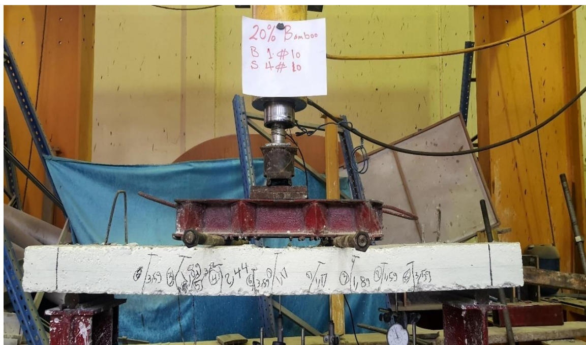
Figure 16. Final Crack patterns for 20% Bamboo Reinforced Slab (S80-B20) %.
