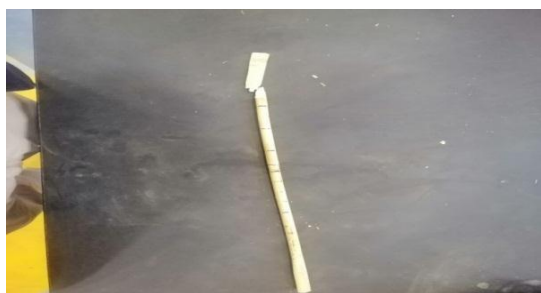
Figure 7. Splitting and Grip Failure (sample-4)
