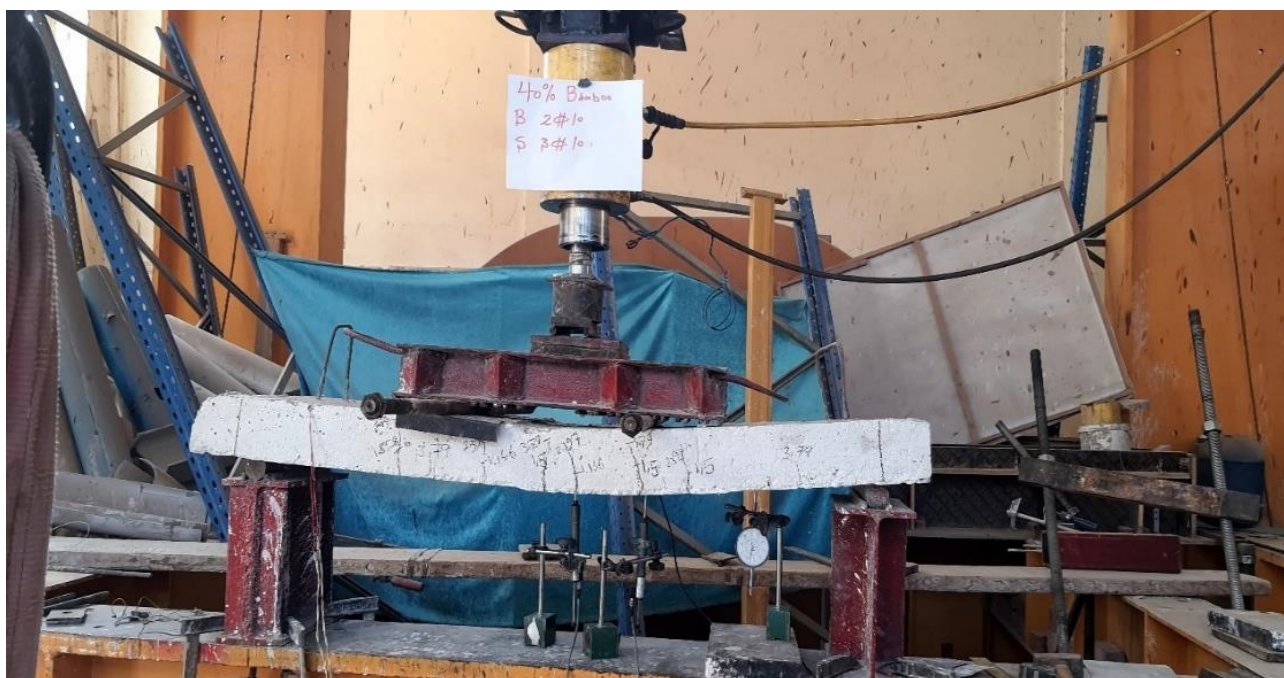
Figure 19. Final Crack patterns for 40% Bamboo Reinforced Slab (S60-B40) %.
