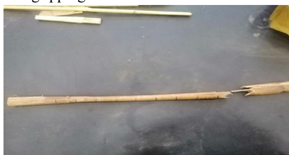
Figure 4. Splitting and Grip Failure (sample-2)
