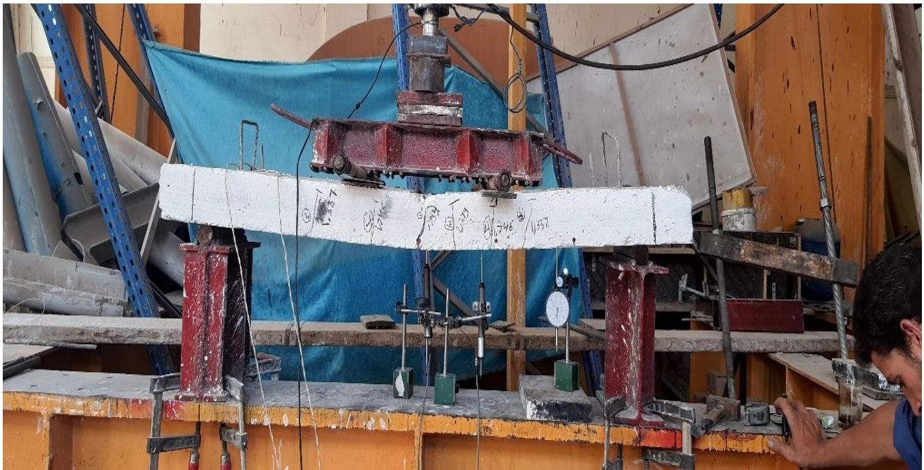
Figure 26. Failure mode for the slab 80% Bamboo (S20-B80) %.
