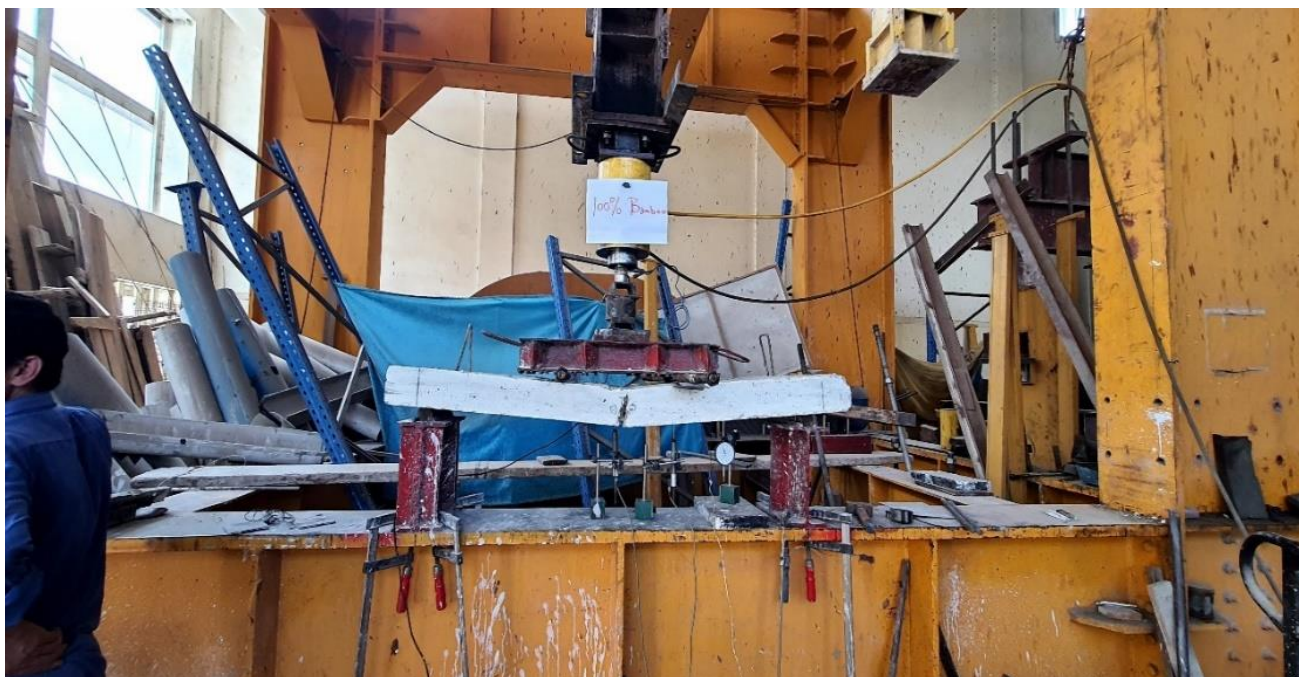
Figure 29. Failure mode for the slab 100% Bamboo (S0-B100) %.
