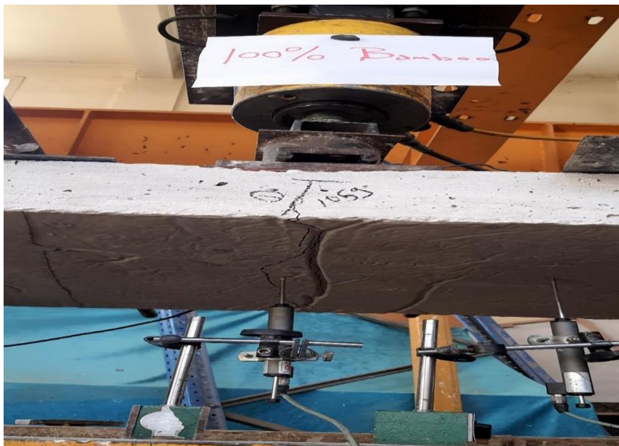
Figure 31. Final Crack patterns for 100% Bamboo Reinforced Slab (S0-B100) %.
