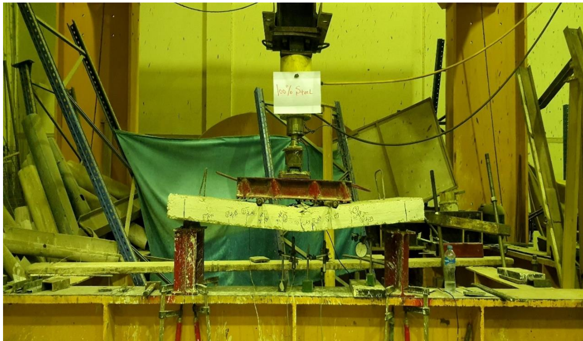
Figure 11. Failure mode for the SLAB 100% Steel (S100-B0) %.
