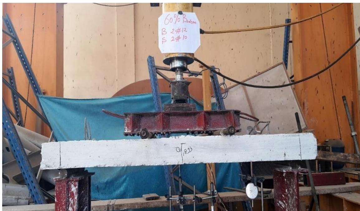
Figure 25. Final Crack patterns for 60% Bamboo Reinforced Slab (S40-B60 12mm) %.
