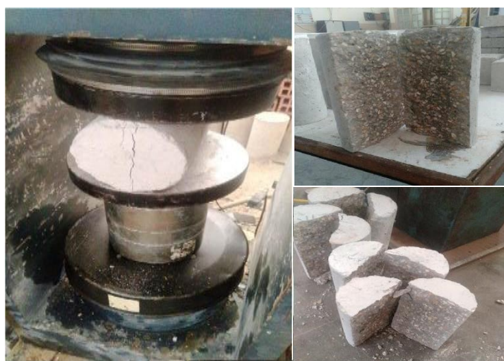
Figure 9. Concrete Tensile Strength Tests Cylinder.
