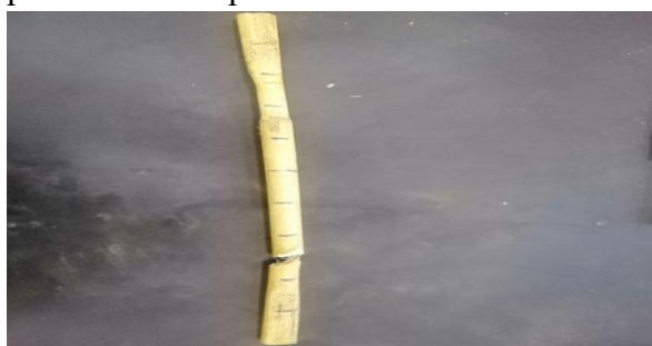
Figure 3. splitting and Grip Failure (sample-1)
