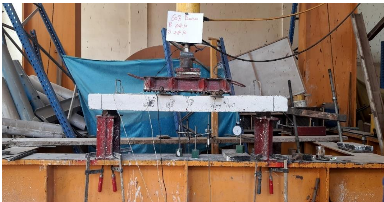
Figure 22. Final Crack patterns for 60% Bamboo Reinforced Slab (S40-B60) %.
