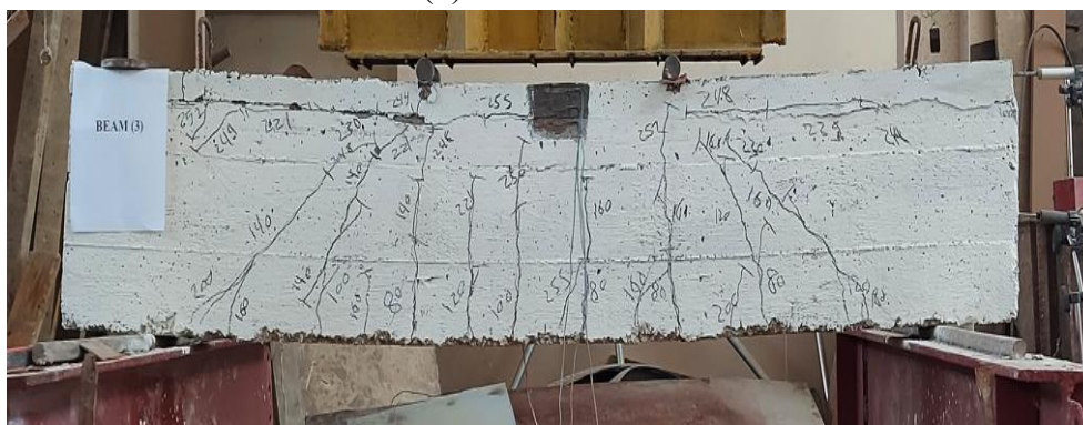
(c) – Failure of B03
