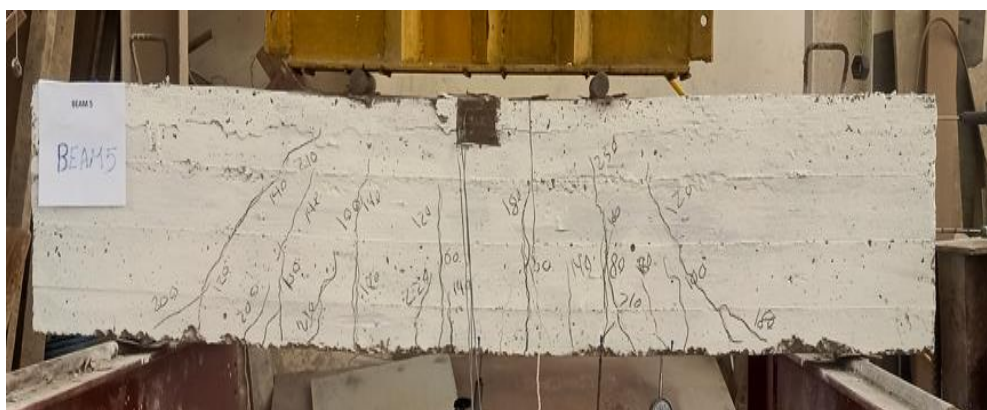
(e) – Failure of B05
