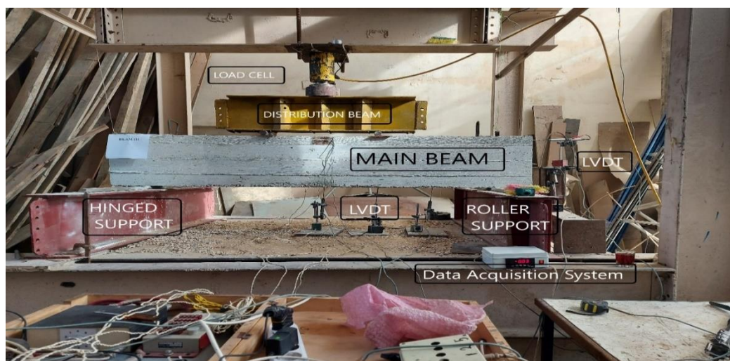
Fig. 3 Test set-up for the beams.
