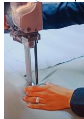
Fig (09) shows the position of operators' fingers and hands while using the Straight knife fabric cutting machine
