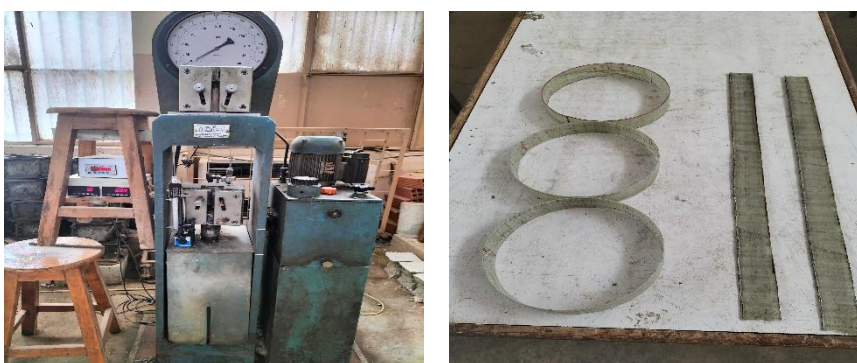
Fig. 2. Tensile test of GFRP coupon samples
