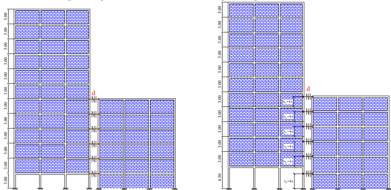
Fig. 9 Seismic pounding between 12-storey pilotis frame and 6-storey infilled-structure (a) Case A or slab-to-slab pounding (b) Case B or slab-to-column pounding
