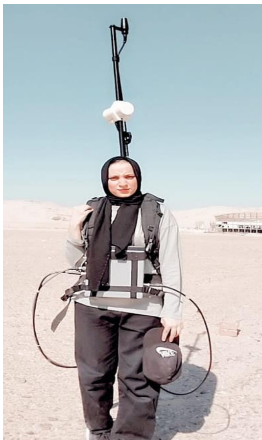
Figure 3: Field photograph of data acquisition using GEM GSM-19 Overhauser magnetometer. The operator was free of any steel or objects that may affect magnetic data.
