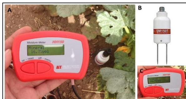
Figure 1. Delta MS 150 moisture meter kit. A. The kit used to measure the soil moisture. B. The SM 150 moisture sensor. C. The HH150 moisture meter (readout unit).
