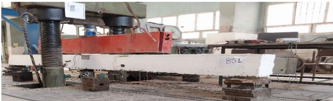
Fig. 2: External instruments and a typical test setup.
