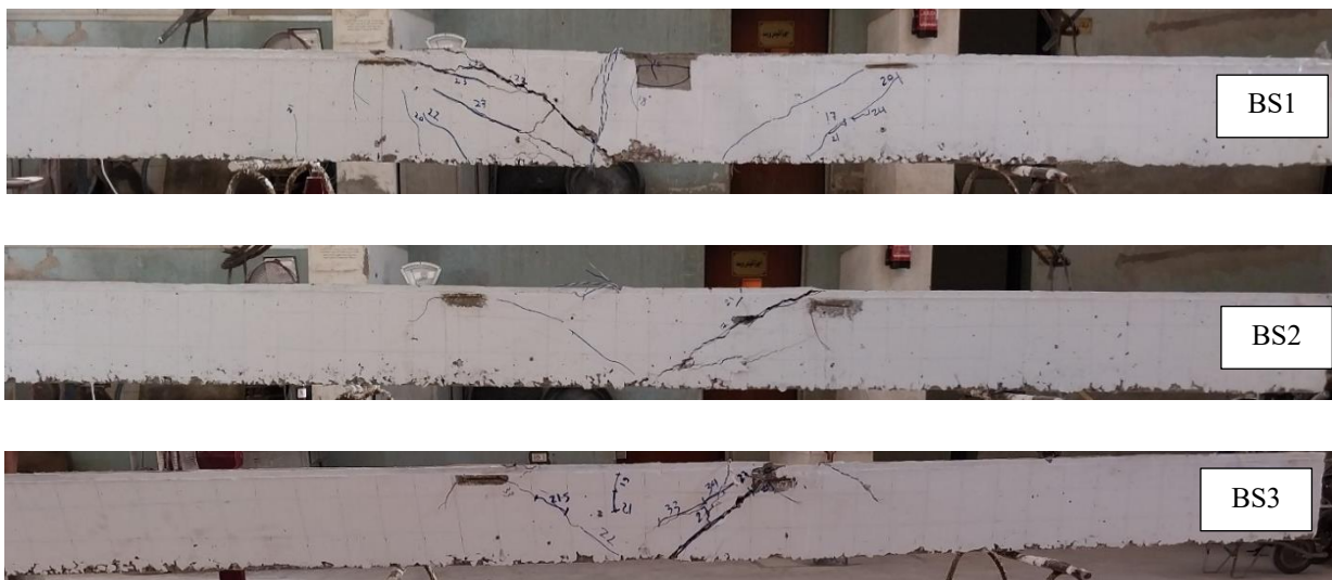
Fig. 3: Cracking patterns and failure modes for test beams BS1, BS2, and BS3, showing diagonal shear failure initiating near the middle support.
