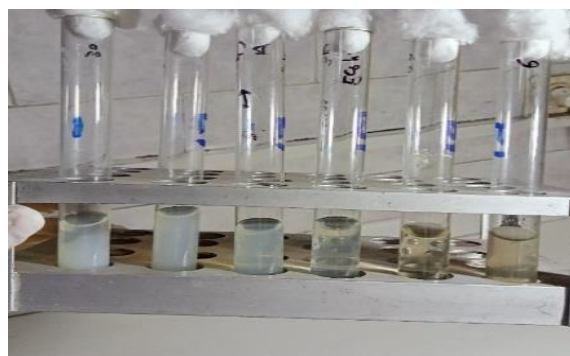
Photo (3): Determination of minimum inhibitory concentration (MIC) of ZnO NPs by nutrient broth media as (1)4.176, (2)1.392,
