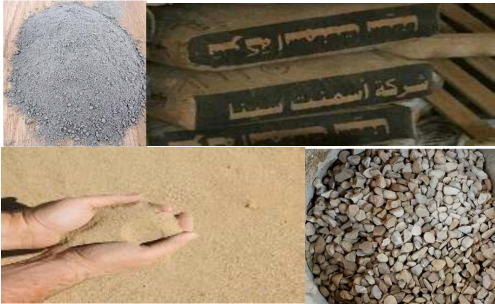
Fig.1. Materials used: Ordinary Portland Cement (OPC), fine and coarse aggregates, potable water, and Steel Slag Powder (SSP).
