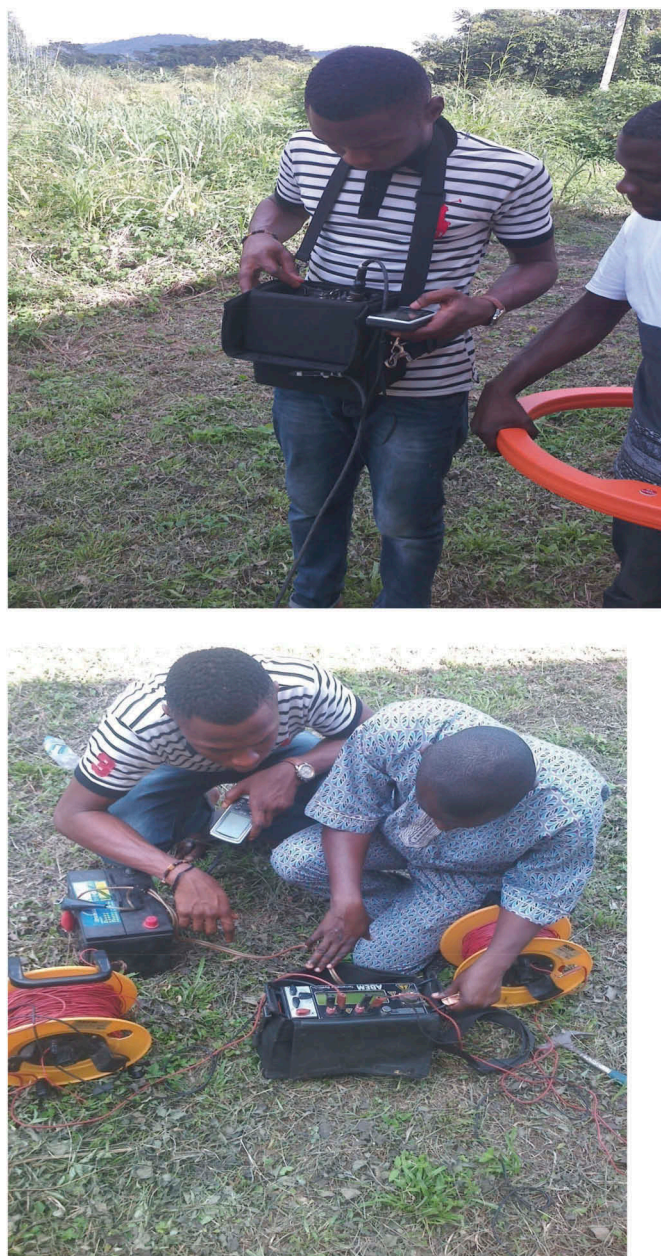
Figure 3. Taking measurement with GEONICS EM 34-3 and Terrameter ABEM SAS 1000.
