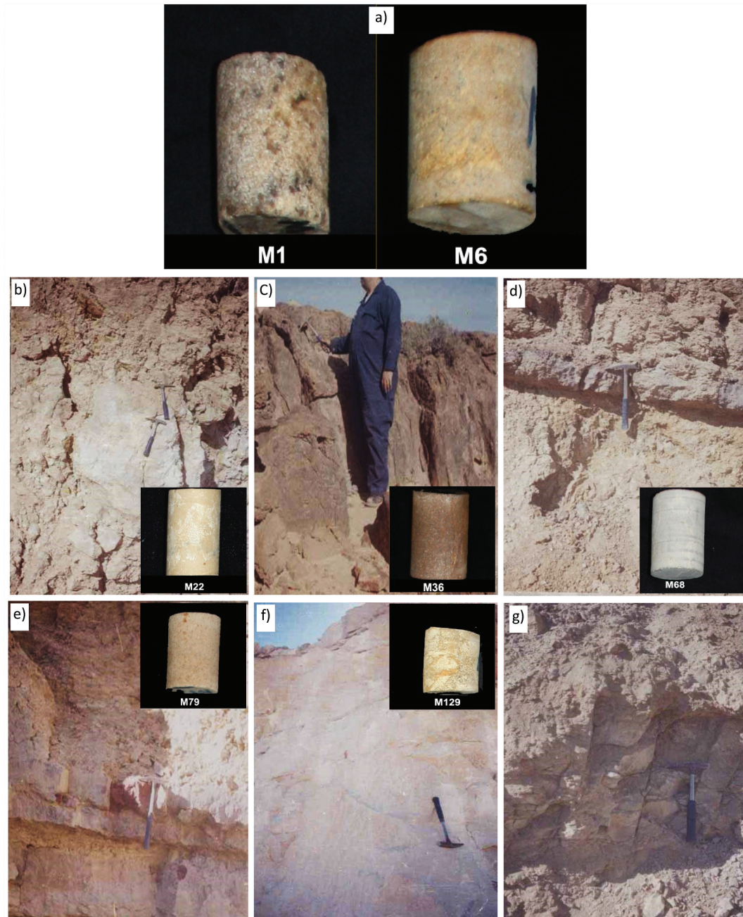
Figure 3. Field photos and plug samples of the Jurassic rocks at Gebel El-Maghara, North Sinai. a) Sandstone (M1) and Limestone (M6) of Mashaba Formation, b) Limestone (M22) of Rajabiah Formation, c) Sandstone (M36) of Shusha Formation, d) Clayey Limestone(M68) of Bir Maghara Formation, e) Sandstone (M79) of Safa Formation, f) Limestone (M129) of Masajed Formation, and g) Shale of Masajed Formation.
