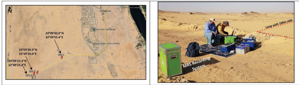
Figure 6. Location of three MRS stations (left) at ~18 km from a known piezometer near Aswan University, Aswan, Egypt. MRS survey at>NNL-1 station (right), Qism Aswan, Aswan, Egypt.
