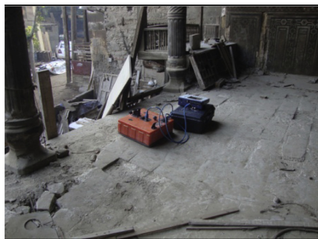
Figure 3 GPR system, Model SIR 3000 (GSSI, USA).
