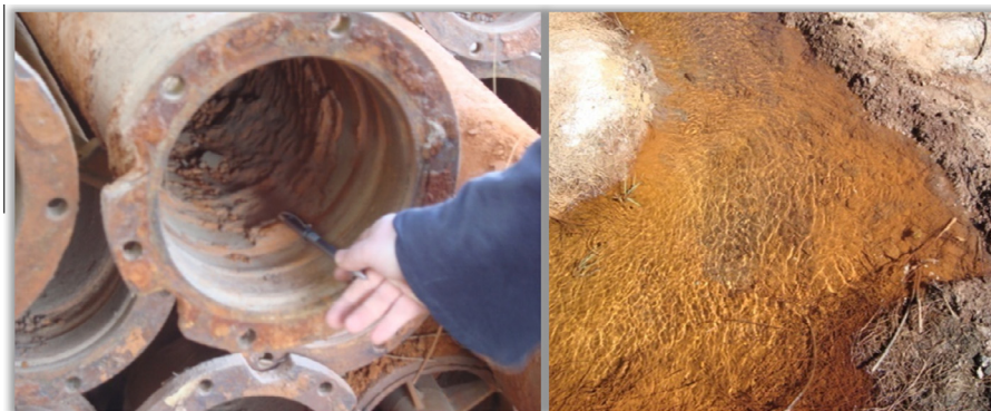
Figure 23 Clogging screens and pipes at El-qulaa drinking water station.
