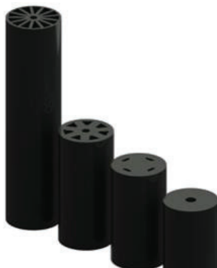
Figure 2. Different fuel grain designs[3].
