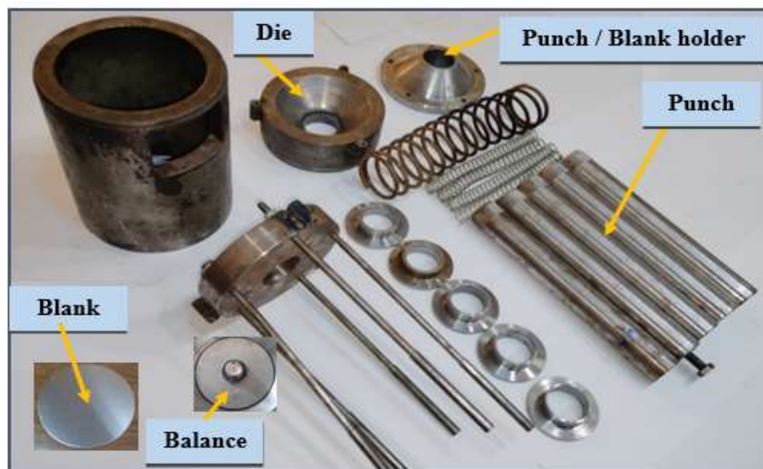
Figure 4 Components of the deep drawing tool and Conical die with Punch / Blank holder
