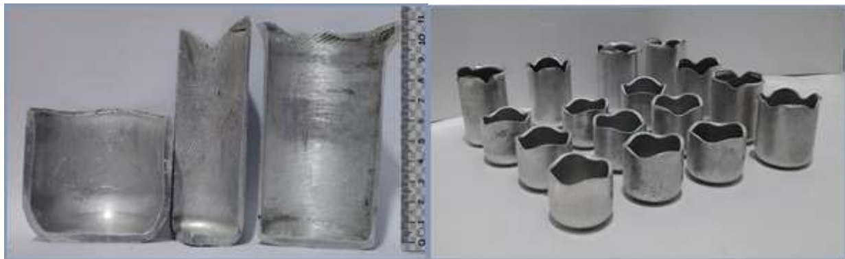
Figure 9 The successful cups and section in some sample at different drawing ratio
