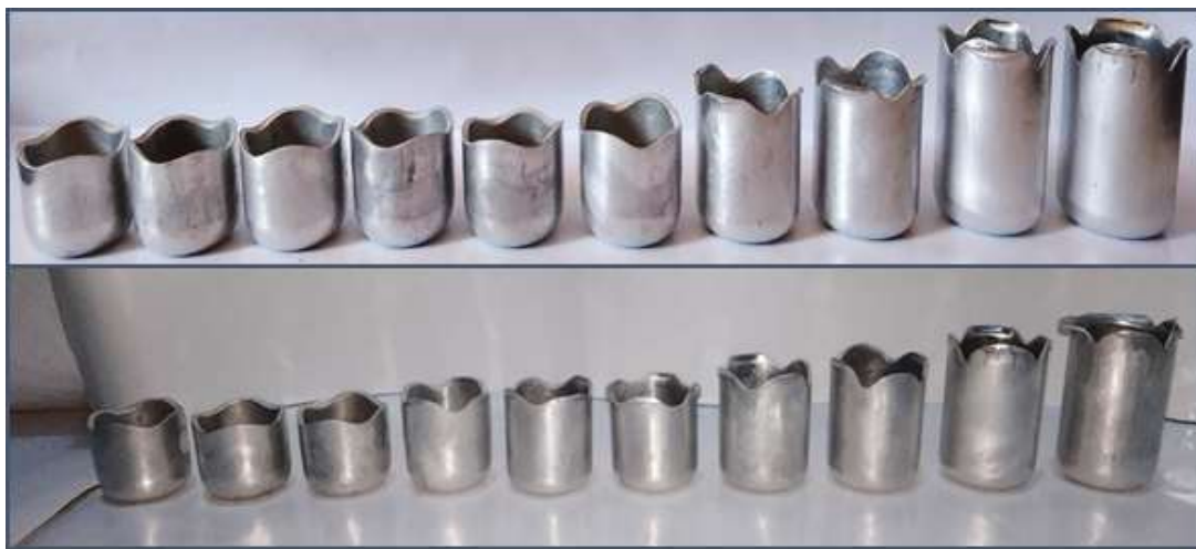
Figure 8 the formed cups for different parameters
