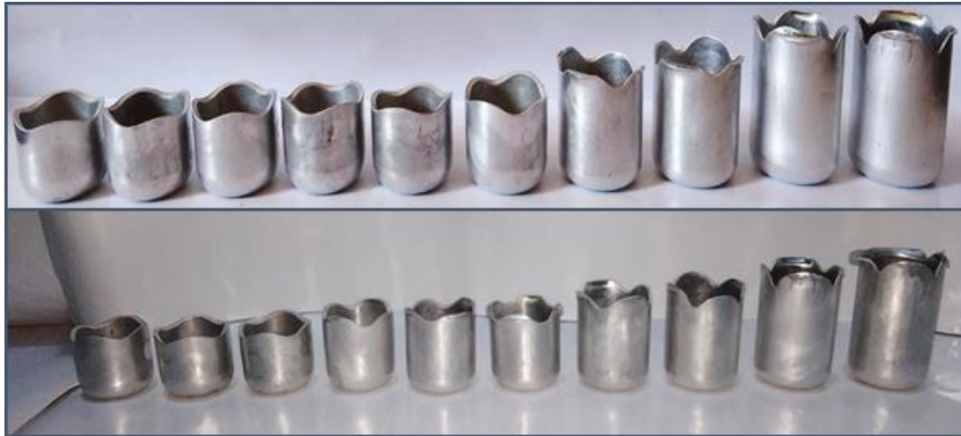
Figure 8 the formed cups for different parameters
