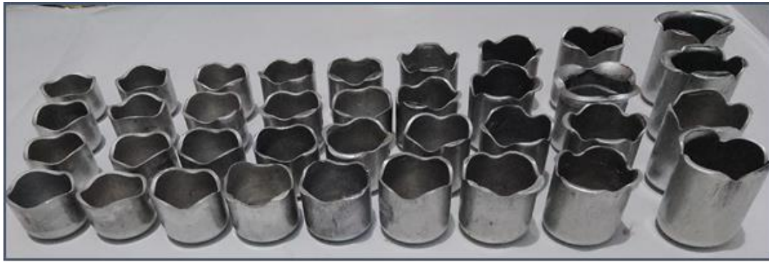
Figure 7 The successful forming cups using by an Innovative Deep Drawing Processes
