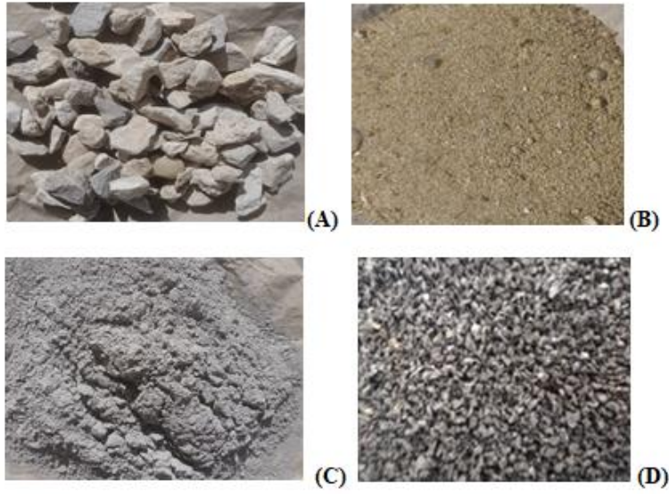
Fig.2. Materials Used in Concrete: (a) aggregate, (b) sand, (c) cement, (d) crumb rubber.
