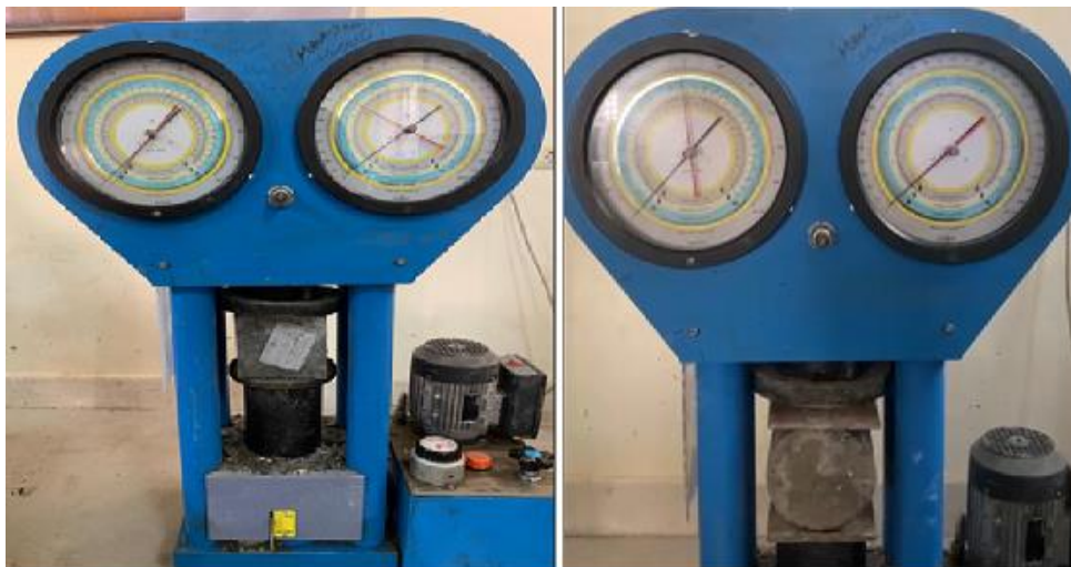
Fig.1. Normal concrete specimen under endurance testing.
