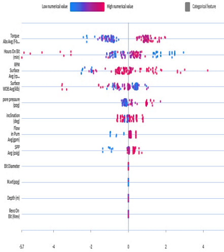
Figure 30: Features Effect for ROP prediction using XGBoost technique before using D-exponent & MSE (Well-2)
