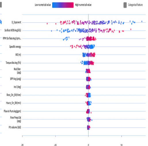
Figure 23: Features Effect for ROP prediction using SVM technique after using D-exponent & MSE (Well-1)
