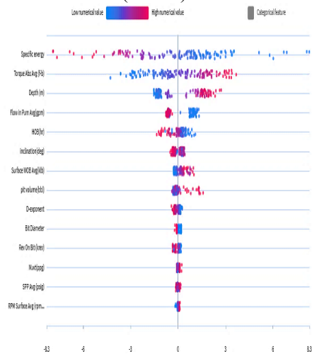
Figure 33: Features Effect for ROP prediction using XGBoost technique after using D-exponent & MSE (Well-3)
