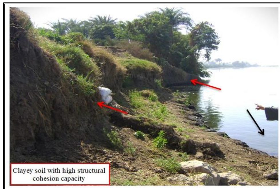
Figure 22. Retention of Structural Cohesion in Clayey River bank Soil during Low Discharge due to Fine Particle Size and Strong Molecular Bonding (Eastern Bank – West of Al-Aqr Village)
