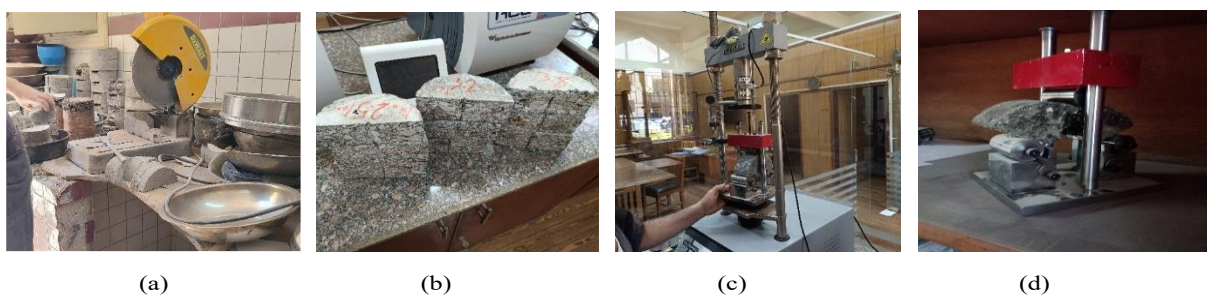
Fig. 8: SCB test at an intermediate temperature of 25C; a) after curing Cut specimen along the center diameter into two semi- circular specimens with notch; b) cut SCB samples with three notch depths; c) sample preparing for SCB test; d) sample after test
