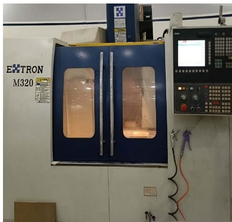
Fig. 1: CNC milling machine (Extron M320 with SINUMERIK 802D SL control) used for the drilling experiments on GFRP specimens.
