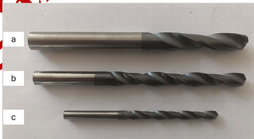
Fig. 4: Solid carbide twist drill bits employed in the study:(a) 10 mm, (b) 8 mm, and (c) 5 mm diameter, all with two-flute geometry and 118°-point angle.
