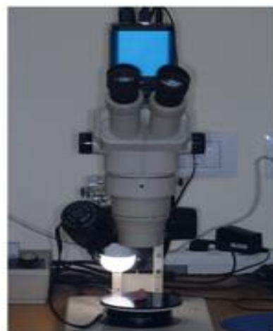
Figure (3): Light stereomicroscope with 5 and 10 folds of magnification (SZ1145TR, Olympus, Japan, 1990)
