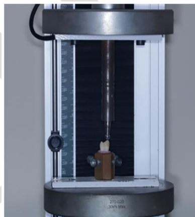
Figure (2): Universal testing machine (5 ST, Tinius Olsen England 2018)
