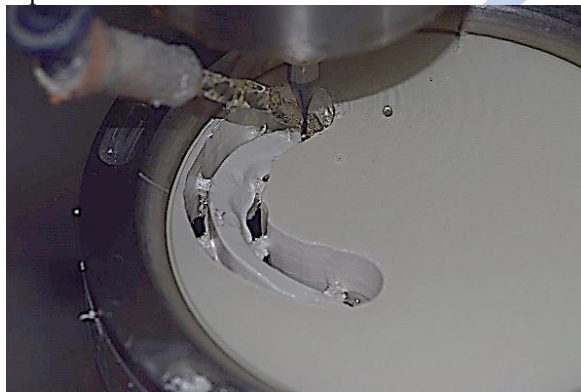
Fig. (2): Milling of PEEK bar.
