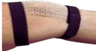
A mesh, featuring anisotropic mechanics and showing the ability to conform to a knee.
