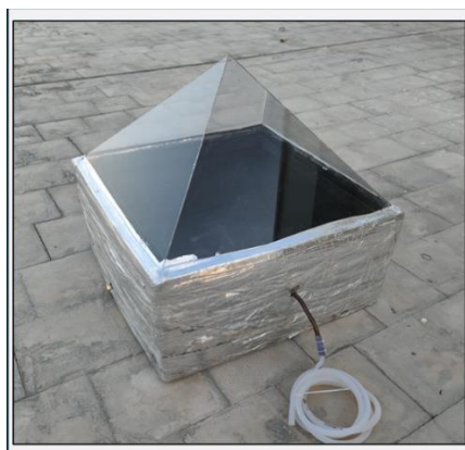
Figure. 2 The photograph of the pyramid solar desalination systems.
