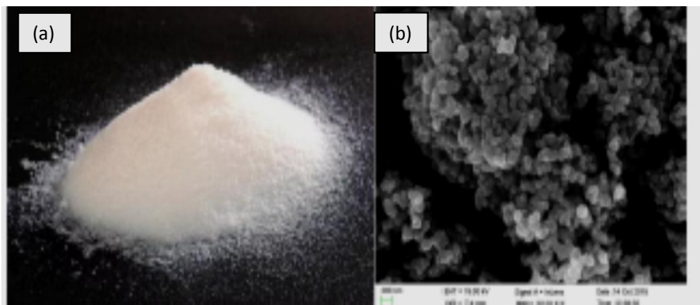
Fig.5. (a) Nano silica, (b) SEM of nano silica
