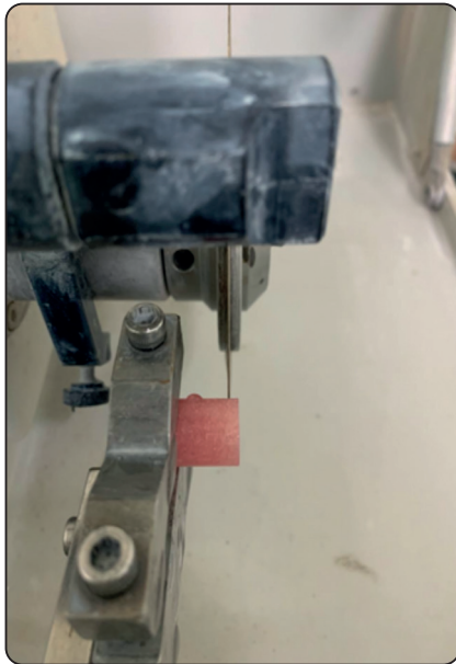
Fig. (1) Sectioning using an IsoMet 4000 micro-saw (Buehler, USA).
