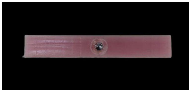
Figure 2: After removing the wire and trimming junctions.
