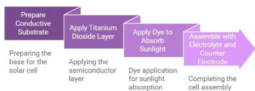
Figure 3: Dye-Sensitized Cell Construction
