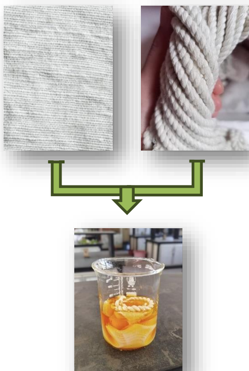
Figure12. Soaking the Fabric in Ferric Chloride
