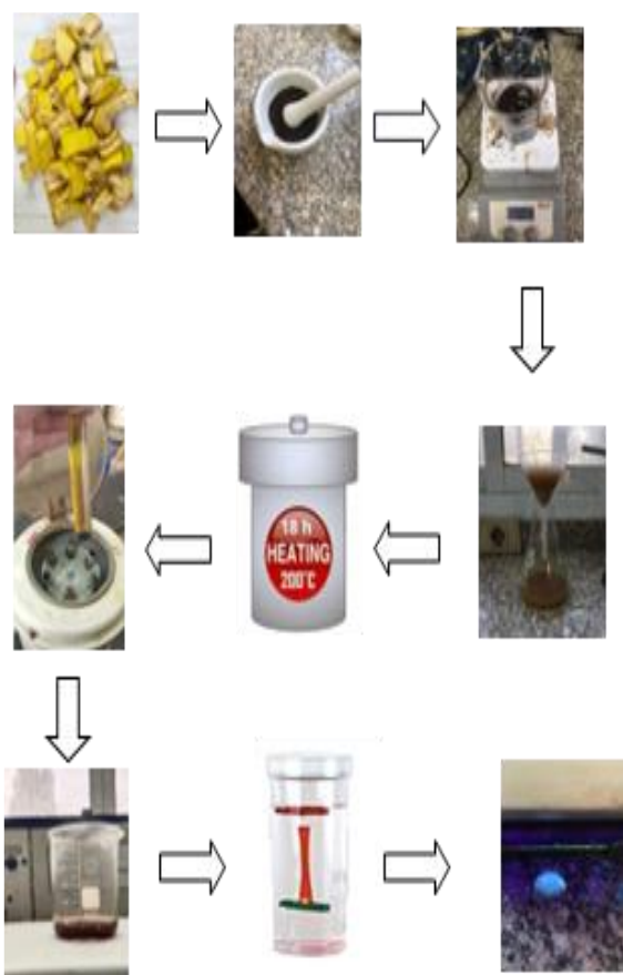
Scheme 1. A Schematic representation of the Synthesis of carbon dots from the banana peels by hydrothermal method.
